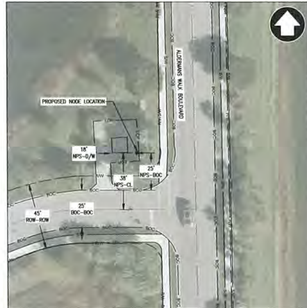
ENLARGED PROPOSED NODE LOCATION PLAN NOT TO SCALE NOTE: LOCATIONS AND DIMENSIONS ARE APPROXIMATE AND BASED UPON AERIAL IMAGES
